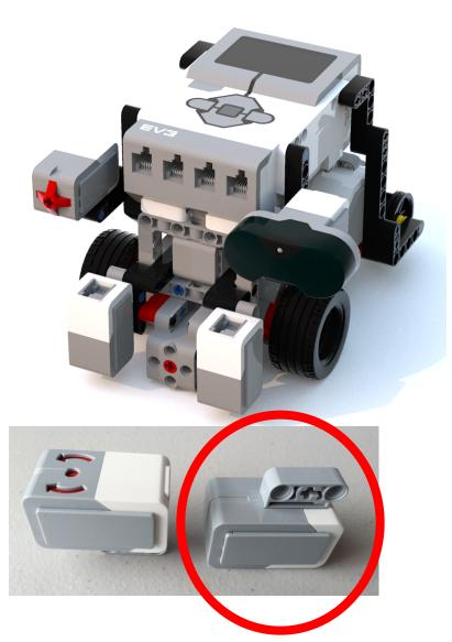
GYRO POSITION FOR A BALANCING ROBOT
