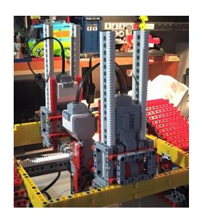
Support structure of Wall-E7 by Marc-Andre Bazergui is made with rack gears
