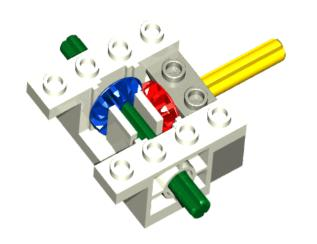
You can use gears to change the direction of motion.
